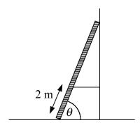
The ladder is prevented from slipping along the ground by a light rope which is attached to the ladder 2m from its bottom end and fastened to the wall so that the rope is horizontal and perpendicular to the wall.
